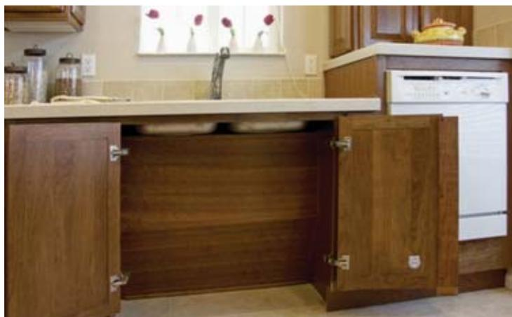
An easily removable decorative panel conceals the sink’s plumbing lines. If pipes are exposed, they should be covered to protect from scalding.
