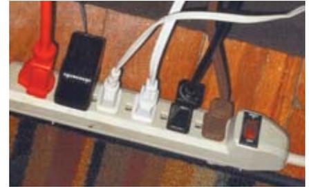
A six-plug power cord adapter replaces old cord gangs. The fused on/off switch will trigger off automatically if overheated.
