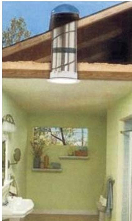
A cross section of a tubular skylight through the roof.
