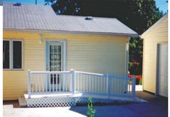
wide and 24'-0" long (8%), and has an open spindle railing on both sides may cost \$25 per square foot or more in the Midwest. That comes to 121 ft<sup>2</sup> including the minimum 5'x5' landing area for a total of \$3,025.
