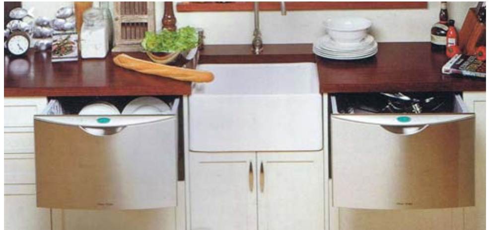
Drawers used to store dinnerware and cooking utensils need to be knob-free and opened using minimum strength. "Intuitive" and "uncomplicated" describe the UD kitchen.
