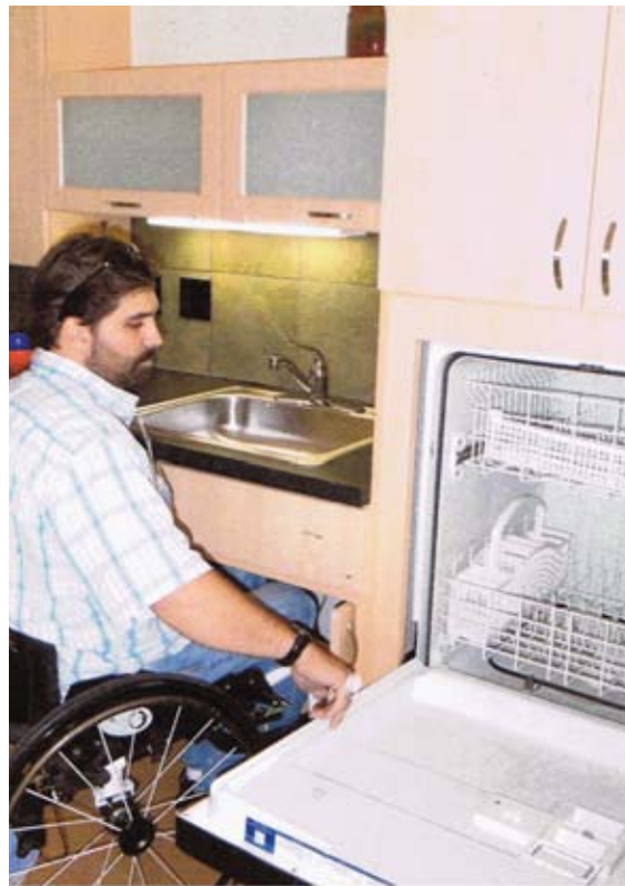
Wheelchair users will find it convenient to use a raised dishwasher adjacent to the sink; under-sink knee space allows for easy access.
